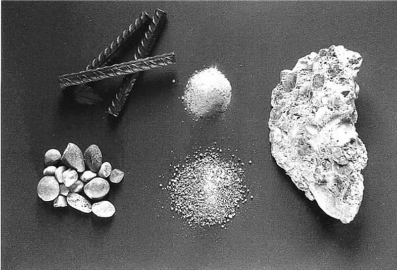
**Fig. 12.10.** Prebroken concrete piece before (*right*) and after (*left* and *centre*) treatment in the discharge vessel of FRANKA 0. Sand and gravel are recovered without degradation. The cement fraction (to the side of the steel pieces) can be baked to produce cement clinker
