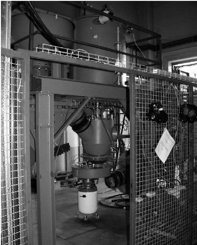
**Fig. 12.11.** View of FRANKA-Stein, a semi-industrial prototype to demonstrate concrete recycling with complete separation of the aggregate at a throughput of up to 1 t/h. The Marx generator is housed in the top cylindrical case
